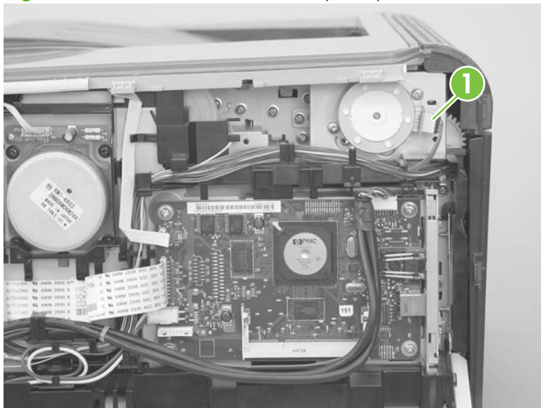
Figure 6-46 Remove the fuser motor (1 of 2)
