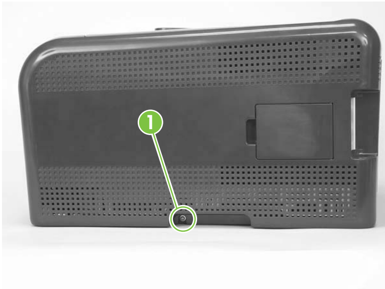
Figure 6-12 Remove the right cover (1 of 4)
