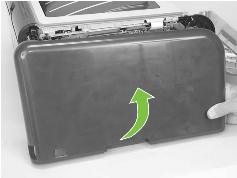
Figure 6-19 Remove the left cover (4 of 4)
