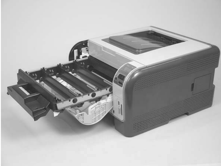
Figure 6-48 Remove the ITB (1 of 9)
