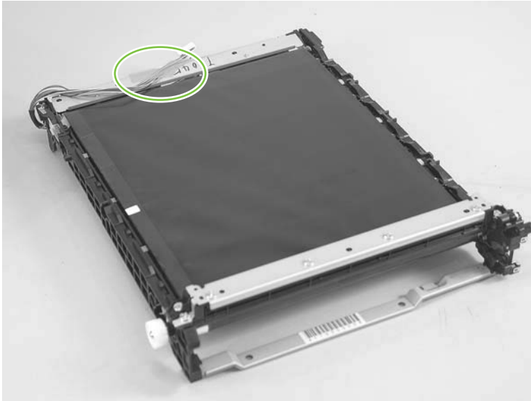
Figure 6-58 Reinstall the ITB (2 of 2)
