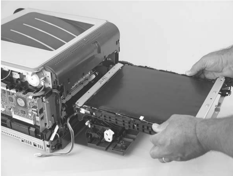
Figure 6-56 Remove the ITB (9 of 9)
