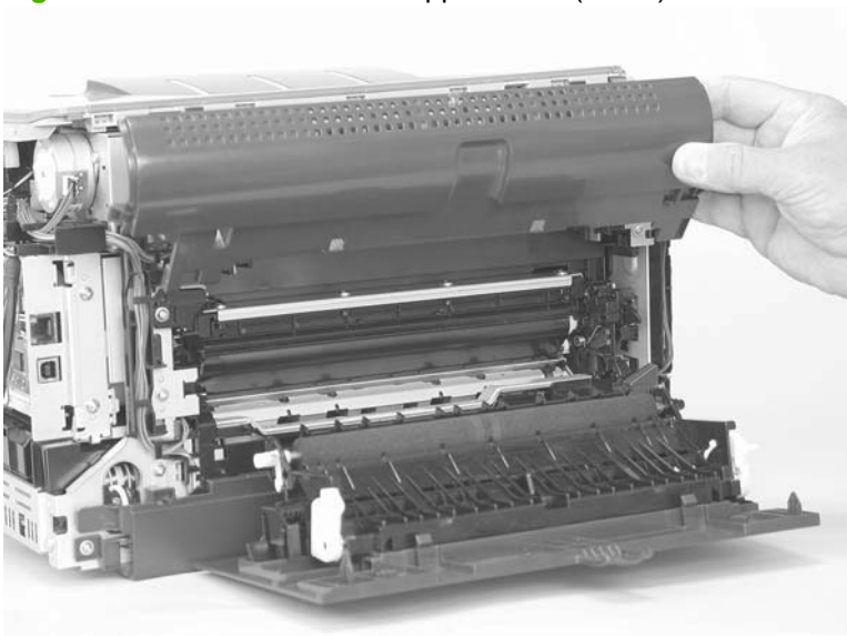
Figure 6-35 Remove the rear-upper cover (2 of 2)
