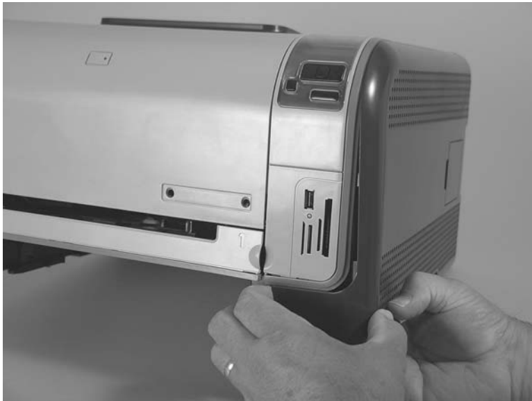
Figure 6-13 Remove the right cover (2 of 4)
